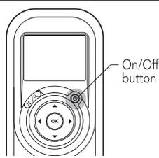
1. Press the On/Off button once. The remote control will start in manual direction control mode.
